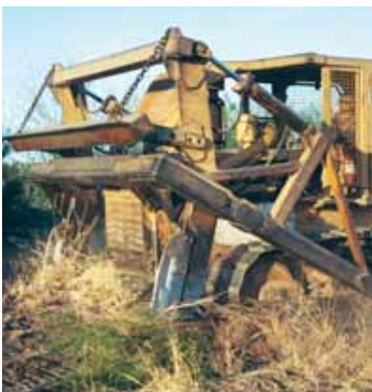
▼ Front-mounted blade plough (Ellrott design)
