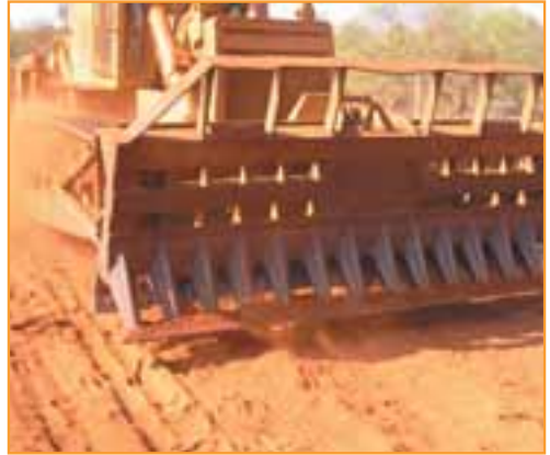
▲ Stick rake with cutter bar.
