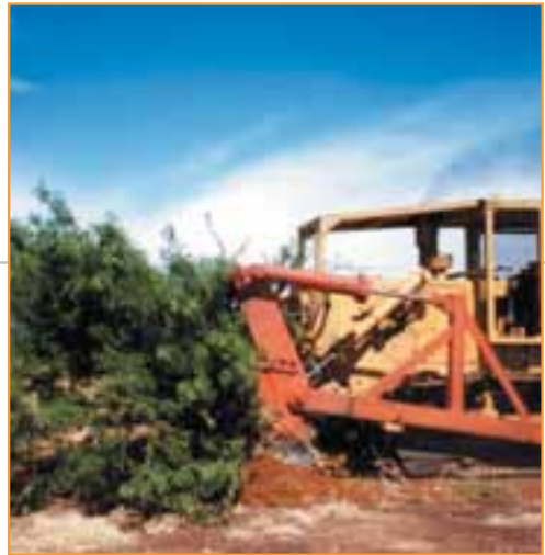
▲ Front-mounted blade plough (Ellrott design).
