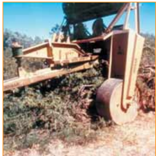
▲ Rear-mounted blade plough (Homan design).
